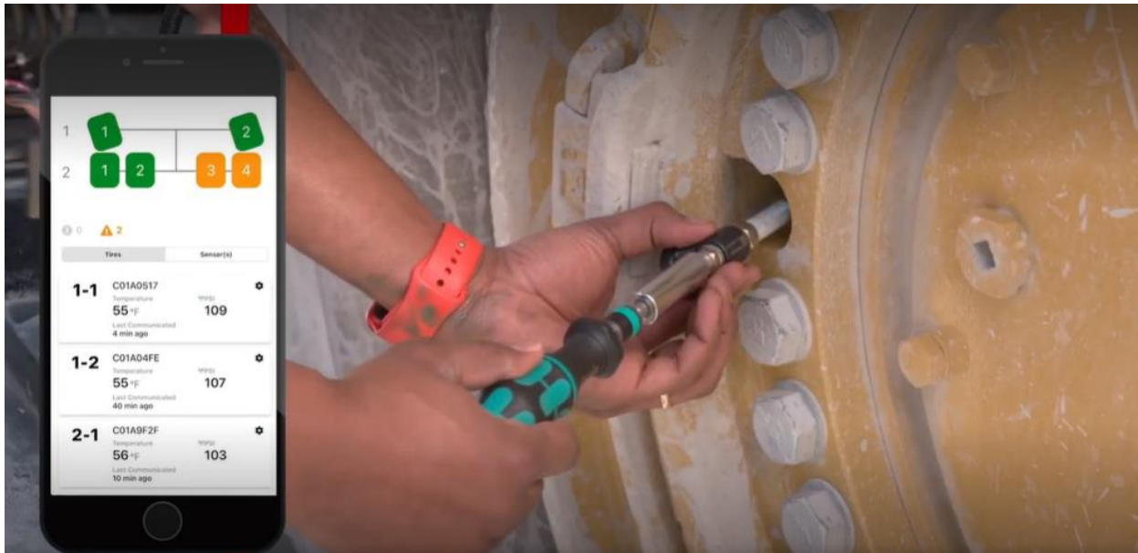
Video 12: Example of Automatic Tyre Pressure Check System - IntelliTire (Bridgestone)
