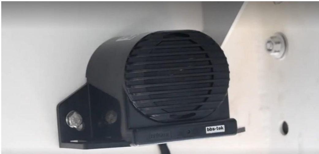
Video 53: Example of self-adjusting white noise reversing alarm – (Brigade)
