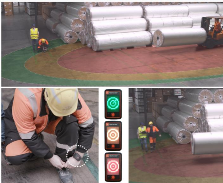
Video 30: Example of Proximity Detection and Alert System – Smart Environment Sensor (Toyota)
