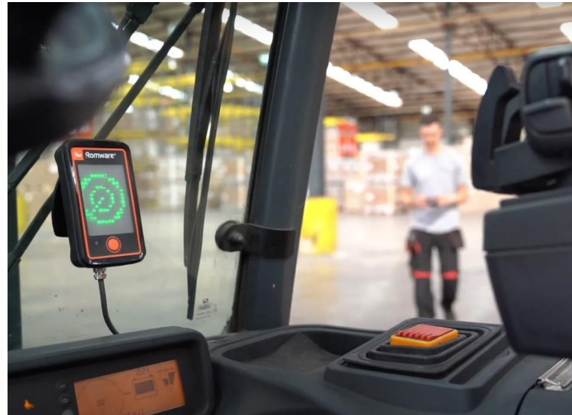
Video 31: Example of Proximity Detection and Alert System (Rombit)
