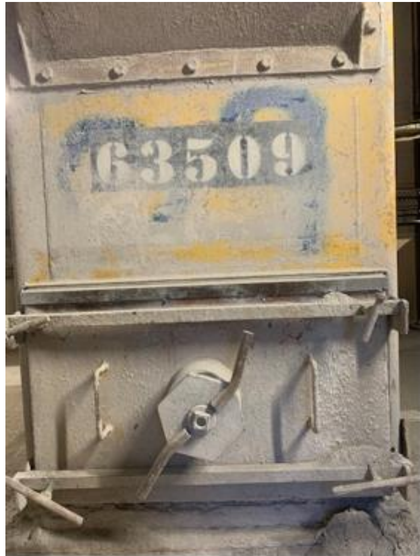
Picture 17: Example of cleaning port at the boot of the bucket elevator
