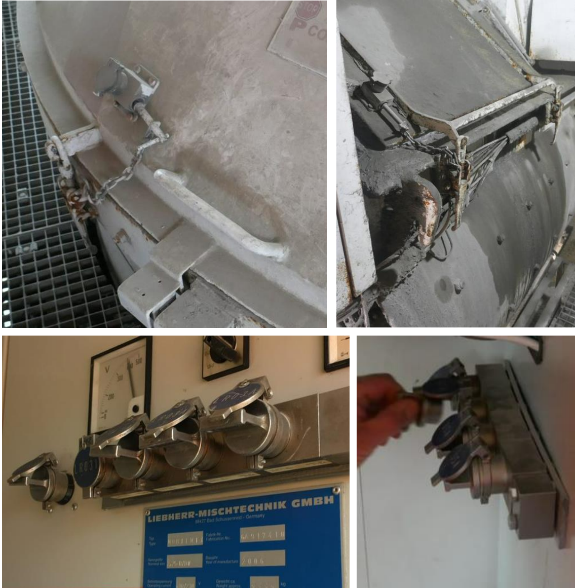
Picture 30: Examples of captive key system
