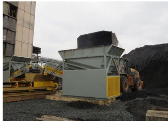
Picture 15: Examples of hoppers fitted with man grid
