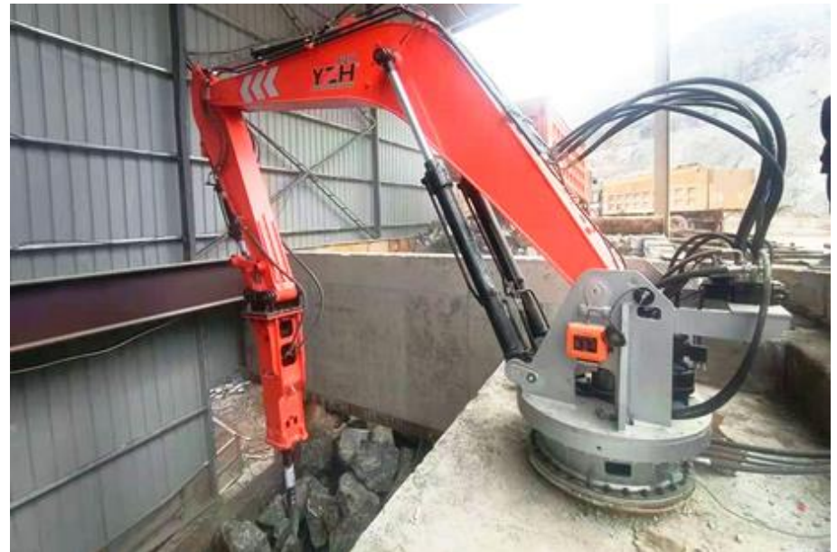
Video 6: Examples of remote-controlled rock breakers for fixed and mobile crushers
