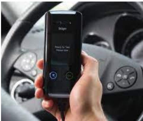
Video 74: Example of Alcohol ignition interlock (Dräger)
