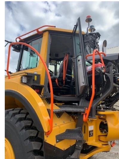
Picture 61: Examples of safe access and guarded working platforms
