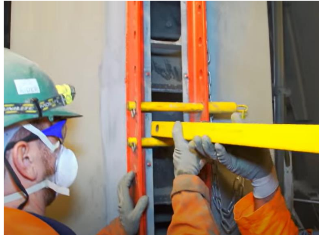
Video 7: Example of mechanical isolation for bucket elevator
