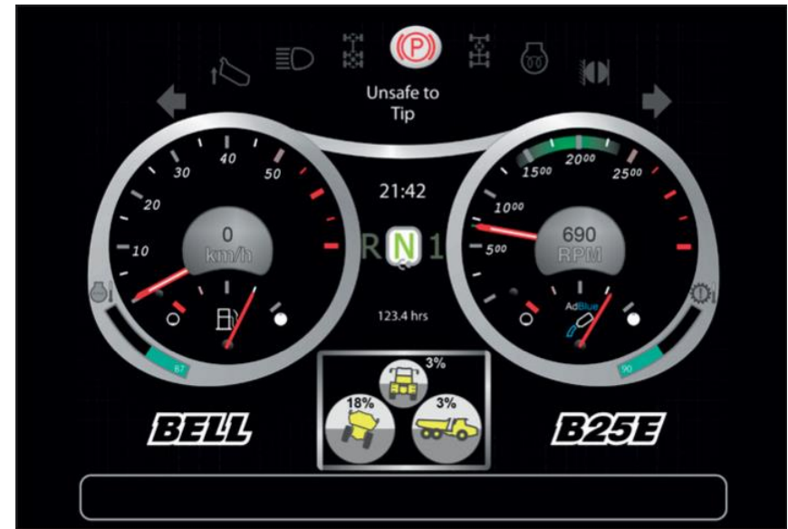
Picture 59: Example of built-in inclinometer (Bell)
