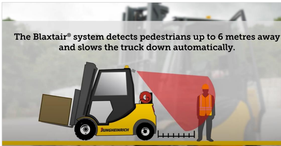
Video 34: Example of Auto brake system using AI for pedestrian detection (Blaxtair / Jungheinrich)
