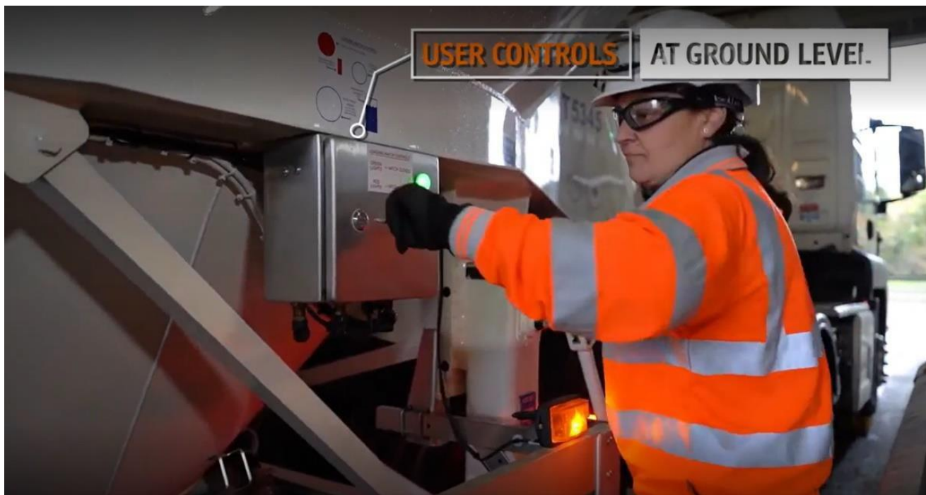
Video 73: Example of Automatic Tanker Hatch System - Auto Loading Lid (Felbinder)
