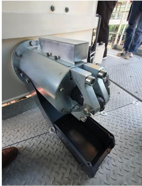
Picture 35: Example of built-in concrete sampling device (Liebherr)
