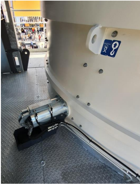
Picture 35: Example of built-in concrete sampling device (Liebherr)
