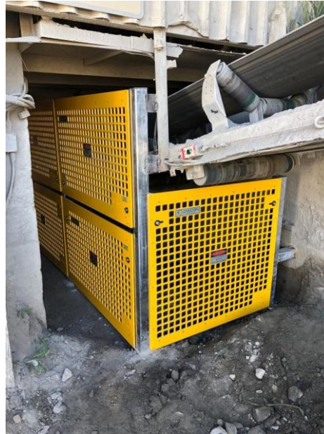
Video 4: Example of Lightweight Machinery Guarding (Diacon)
