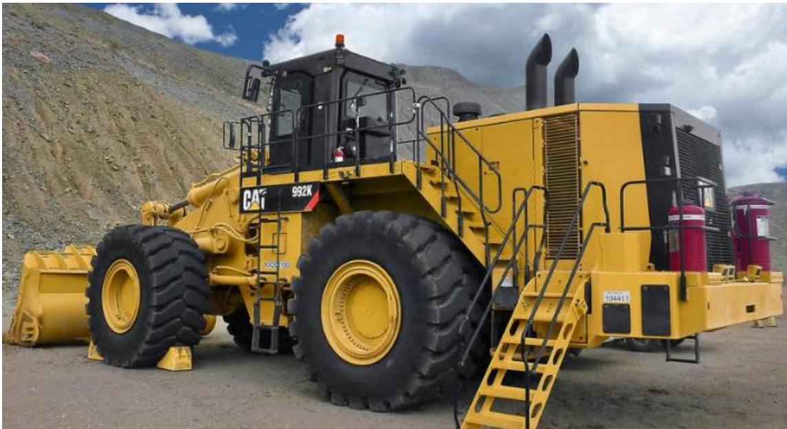
Picture 57: Examples of safe access stairs (instead of ladders) on large quarry equipment
