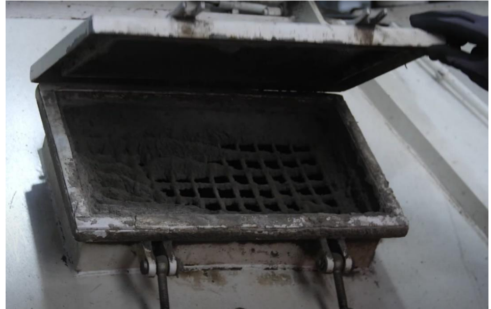
Picture 32: Example of mixer discharge point and inspection hatch guarding
