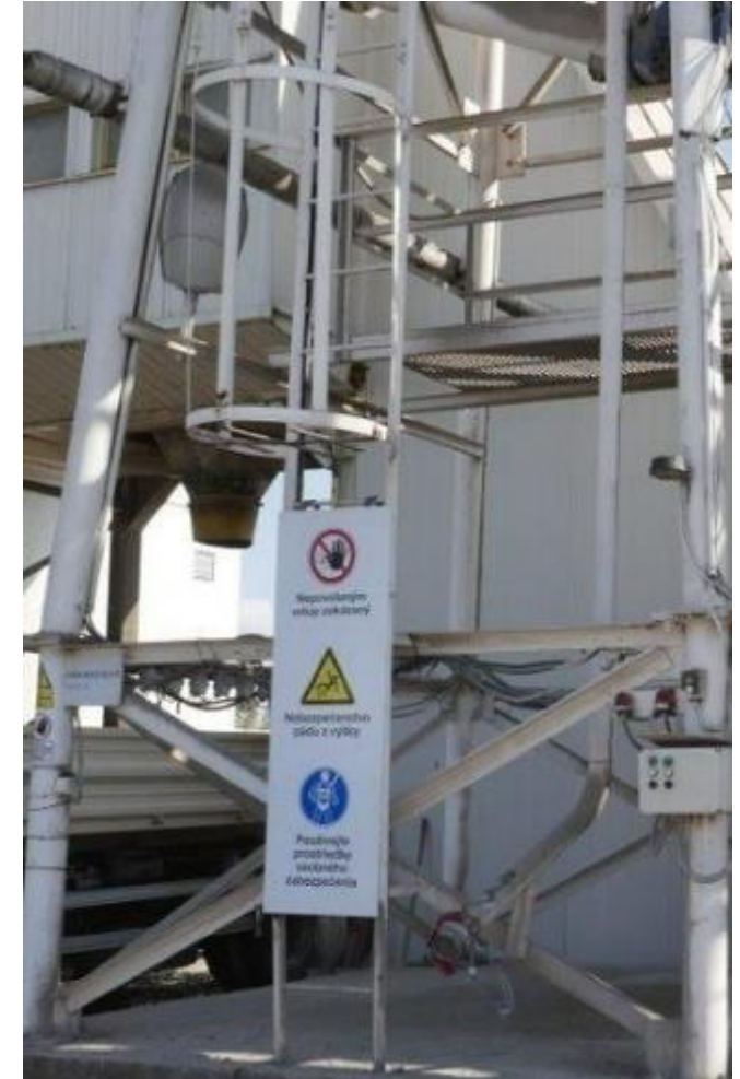
Picture 20: Example of ladder restriction - padlock key is required to access the ladder
