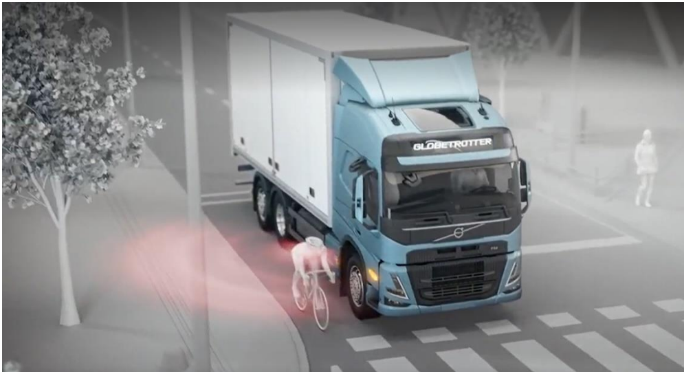
Video 49: Example of Side Collision Avoidance System - Side Collision Avoidance Support (Volvo)
