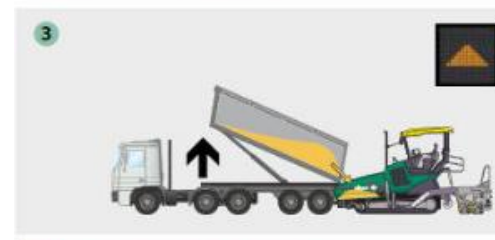
Video 38: Example of Traffic Light System - PaveDock Assistant (Wirtgen Group)
