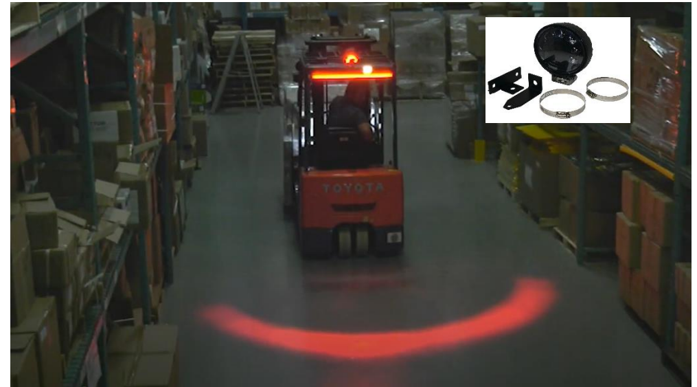
Video 27: Example of Warning Light – Arc Red Light System (Toyota)
