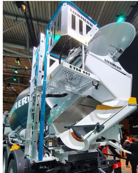
Picture 81: Example of guarded crows nest platform with self-closing anti-fall safety bar – Guardrail is designed to prevent drivers standing on the middle rail
