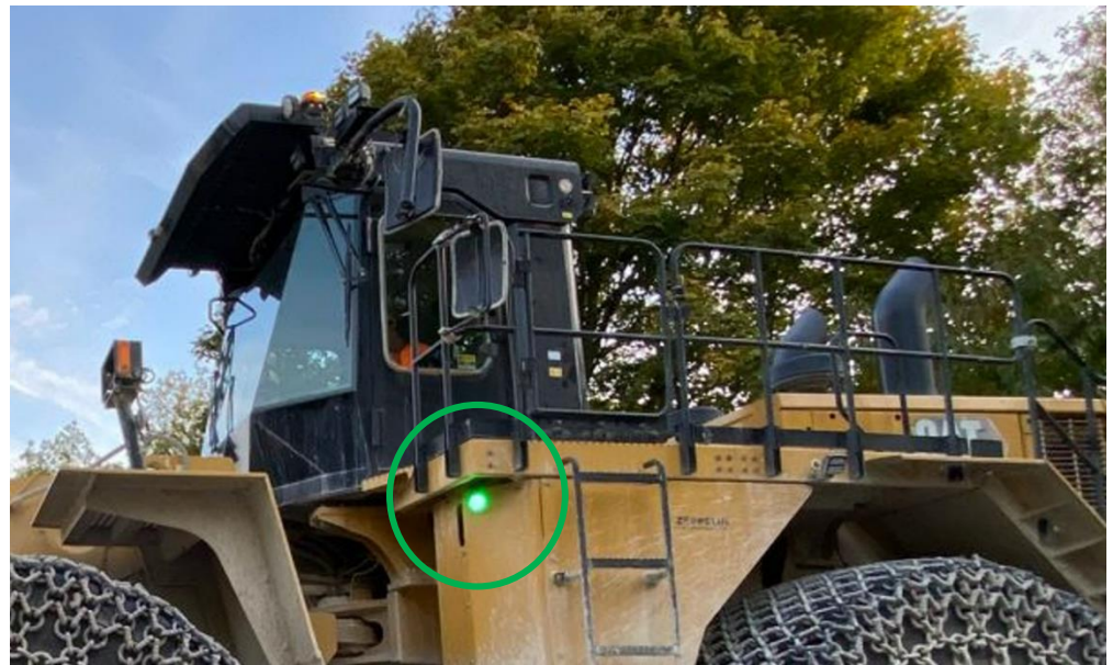
Picture 58: Example of high-visibility seat belt and seat belt use indicators – visual and audible dashboard alarm; a green light on the outside to indicate whether the safety belt is fastened
