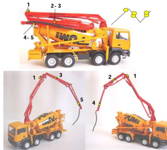
Picture 85: Example of Powerline Proximity Alert System (Sky NG Radio)
