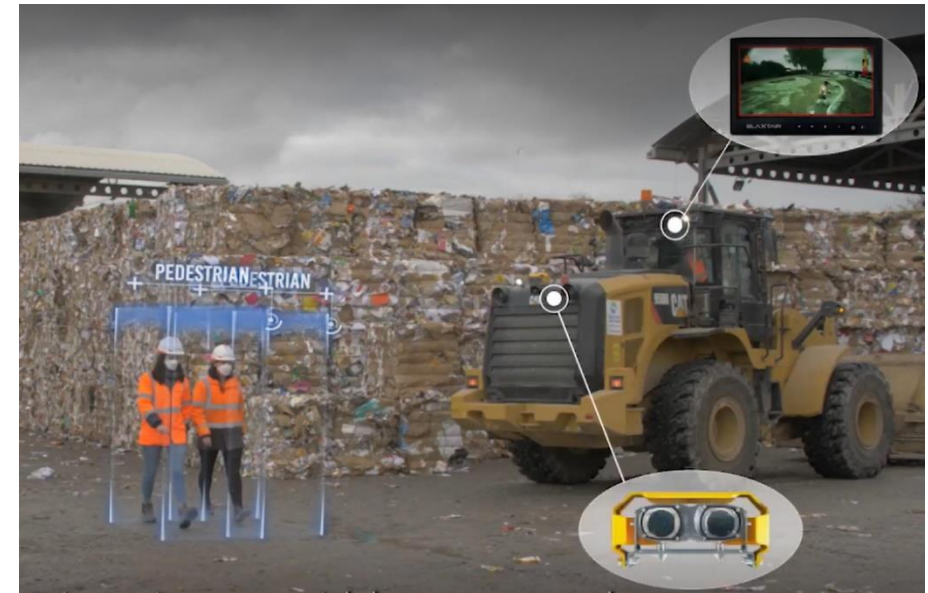
Video 18: Example of proximity detection system - Pedestrian Detection using AI (Blaxtair)
