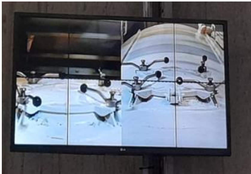
Picture 39: CCTV with a fixed crosshair that is visible to drivers via a display screen
