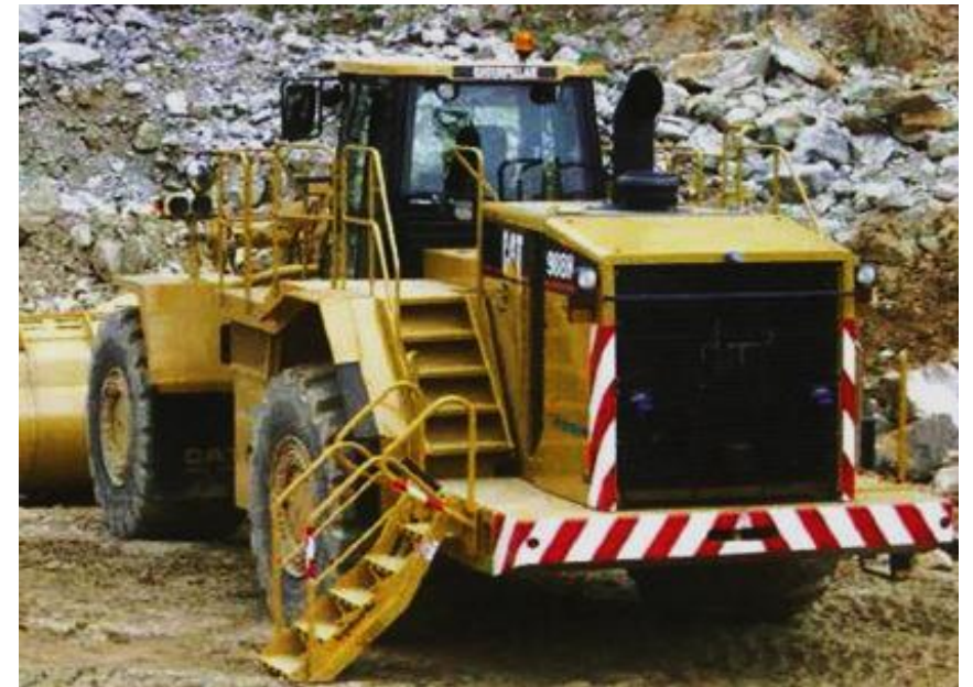
Picture 57: Examples of safe access stairs (instead of ladders) on large quarry equipment
