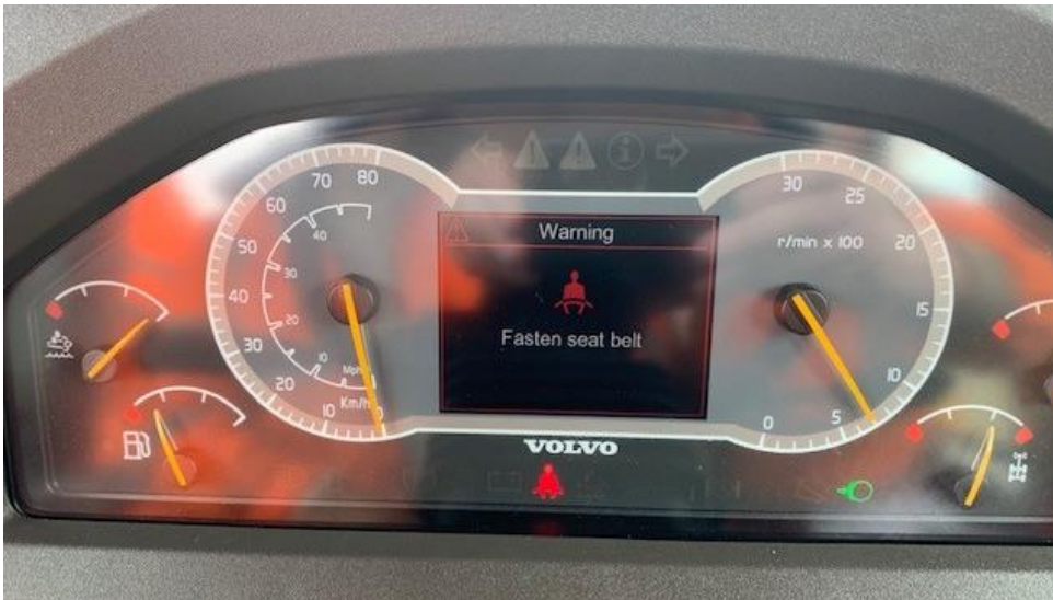
Picture 64: Examples of visual and audible warning signs (seat belt, parking brake)
