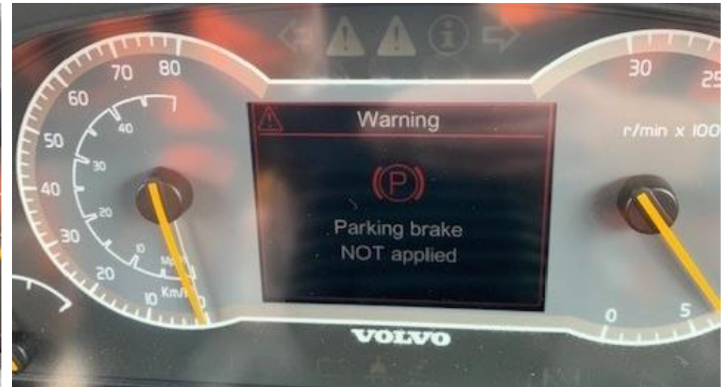
Picture 64: Examples of visual and audible warning signs (seat belt, parking brake)
