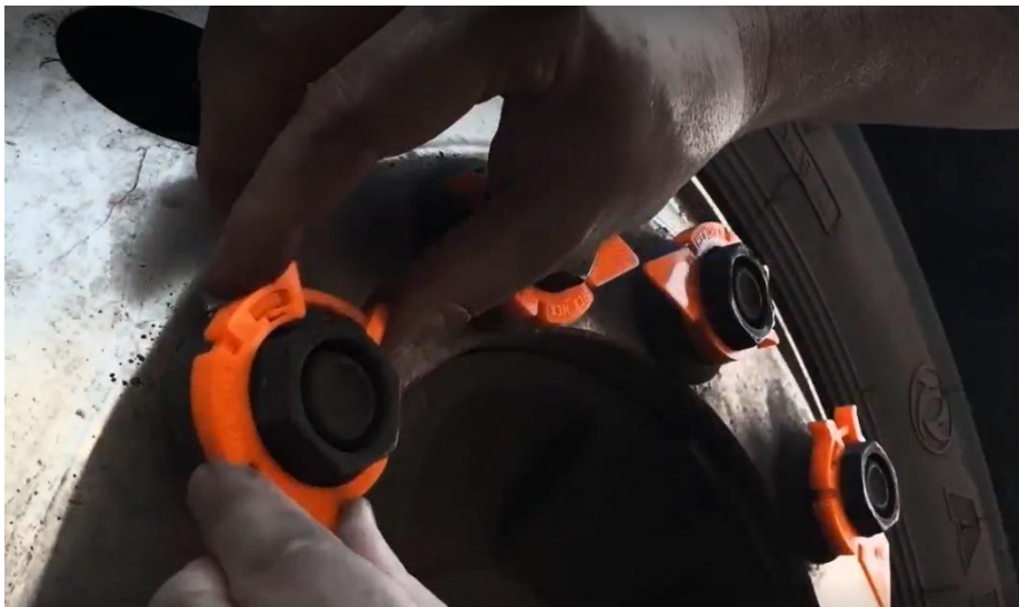
Video 47: Example of adjustable Wheel Nut Indicator (HexChex)
