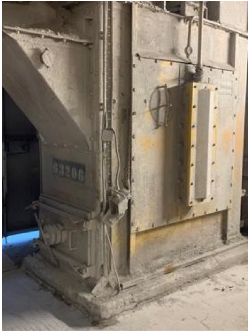
Picture 17: Example of cleaning port at the boot of the bucket elevator
