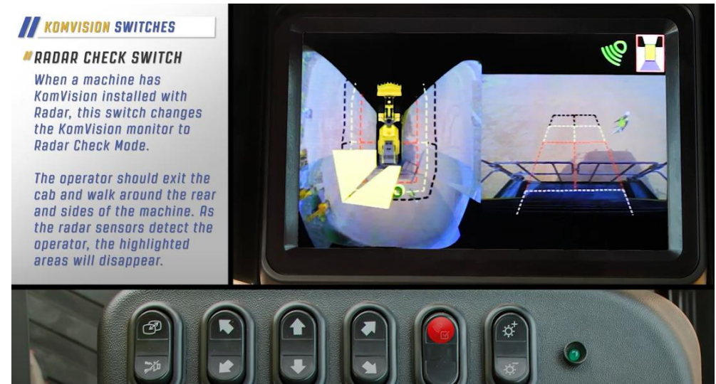
Video 16: Example of proximity detection system - Komvision (Komatsu)
