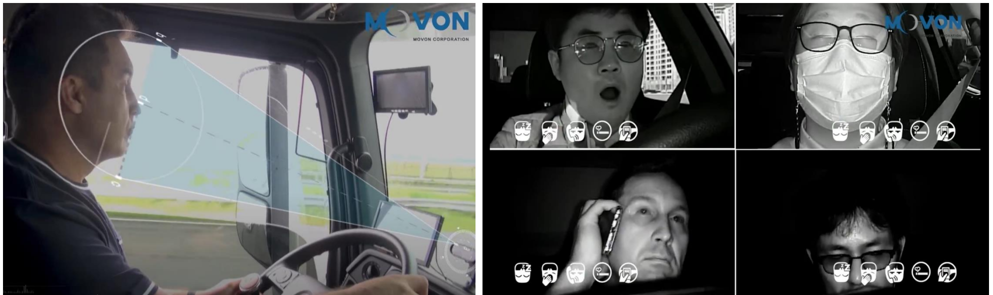
Video 65: Example of Driver Fatigue Monitoring System (Movon)
