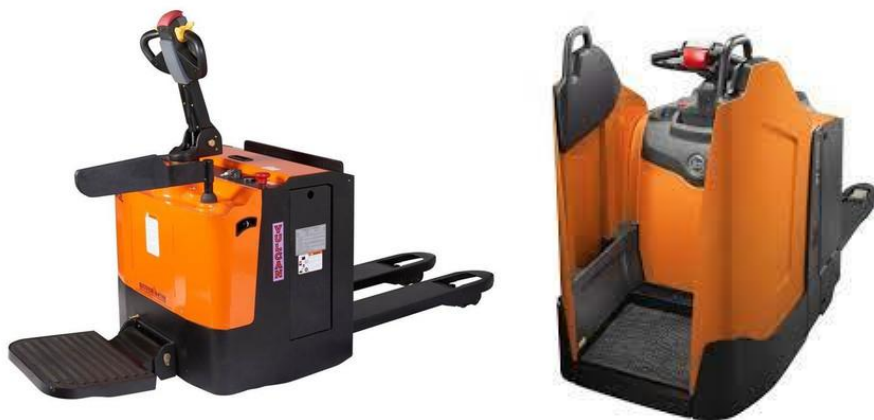
Picture 68: Examples of pallet trucks with side protection
