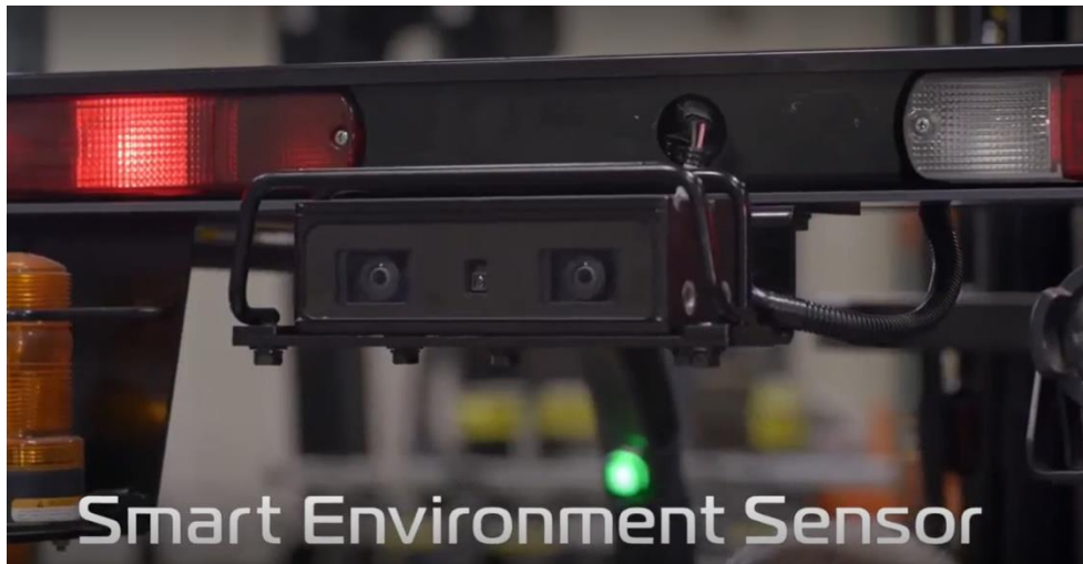
Video 30: Example of Proximity Detection and Alert System – Smart Environment Sensor (Toyota)
