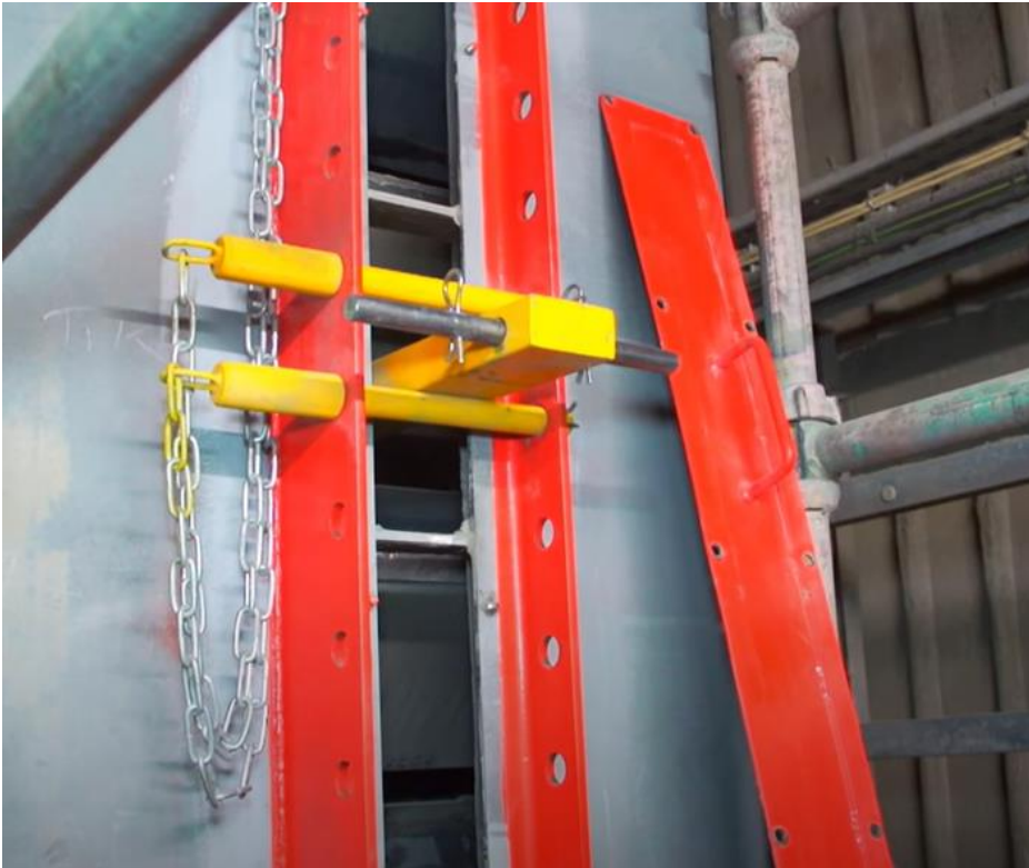
Video 7: Example of mechanical isolation for bucket elevator
