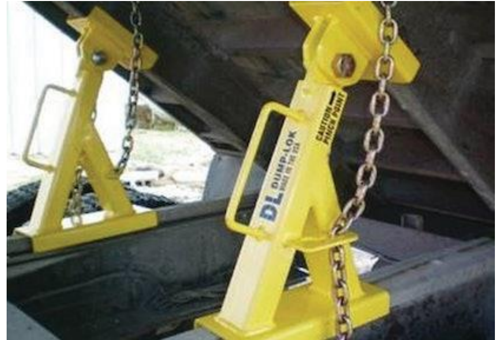
Picture 53: Examples of high visibility locking brackets / body props
