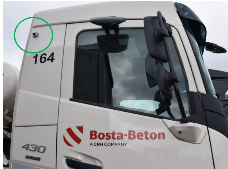
Video 52: Example of 360° Blind Spot Camera System with Bird-eye view feature (Brigade)
