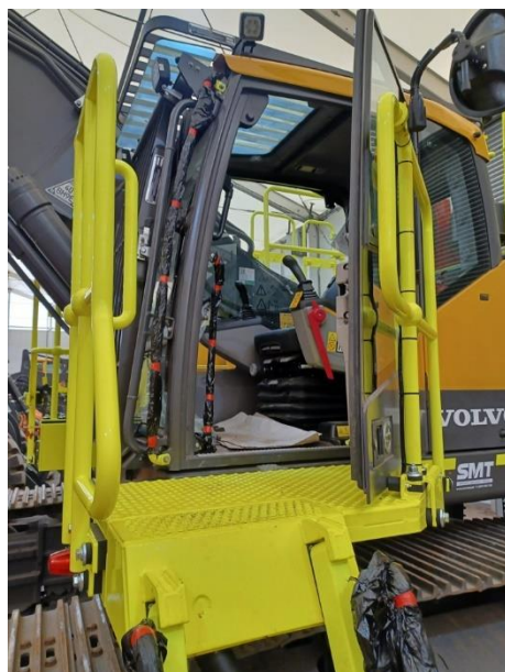
Picture 52: Examples of Hi-Viz marking of handrails on mobile plant to aid visibility and reduce the potential for falls from height
