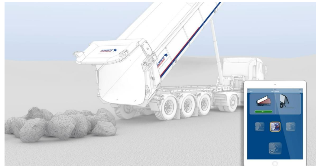
Video 66: Example of remote-controlled tailgate (Schmitz)
