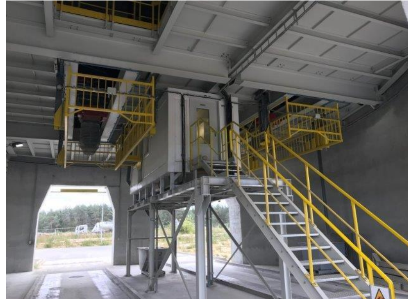
Picture 37: Examples of truck loading mechanisms with safe access
