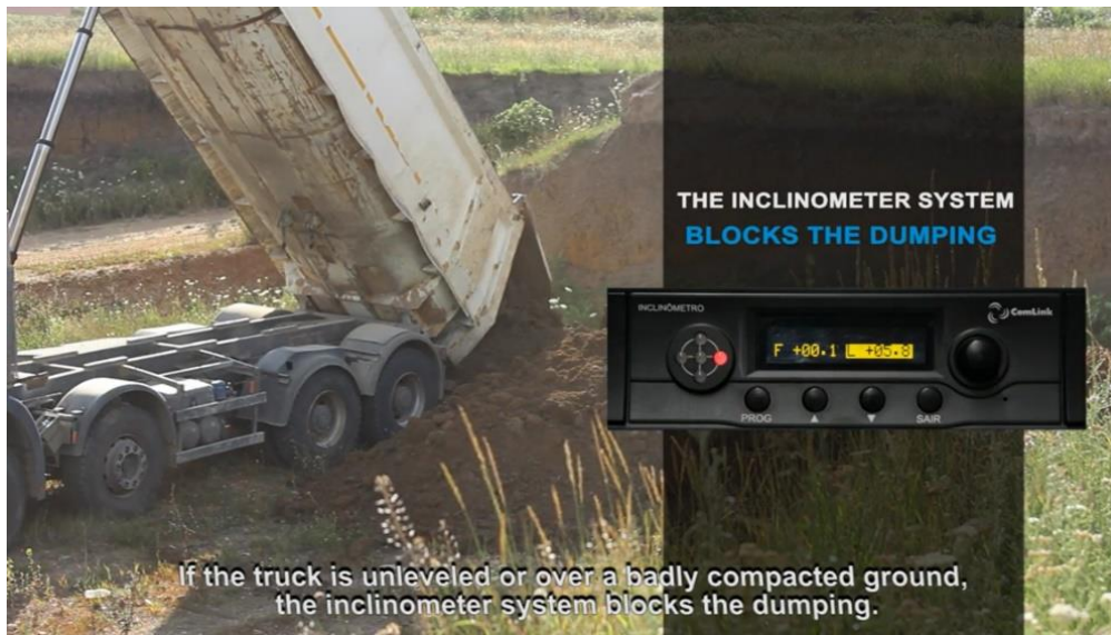
Video 58: Example of Active Inclinometer for tipper trucks – System warns the driver and stops tipping
