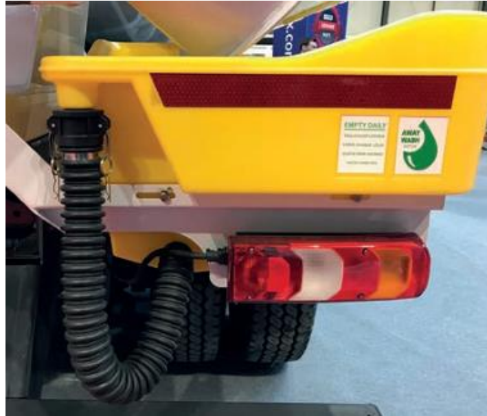
Video 60: Example of chute washout system - Away Wash (Jonesco)
