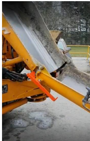
Video 59: Example of Finger Trap Prevention Device for folding type chutes
