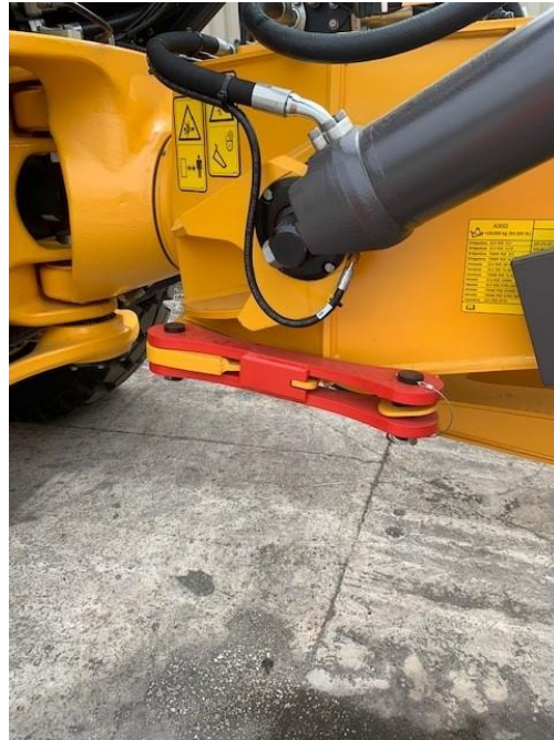
Picture 53: Examples of high visibility locking brackets / body props
