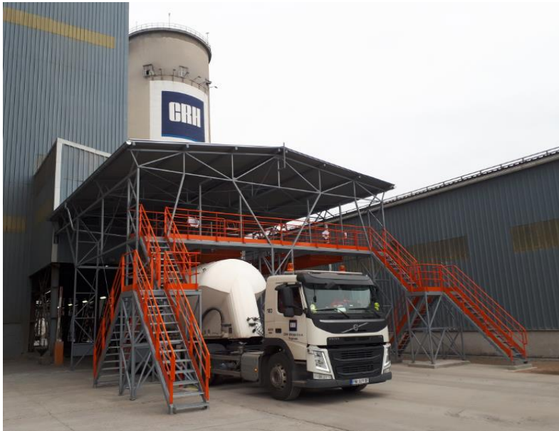
Picture 37: Examples of truck loading mechanisms with safe access
