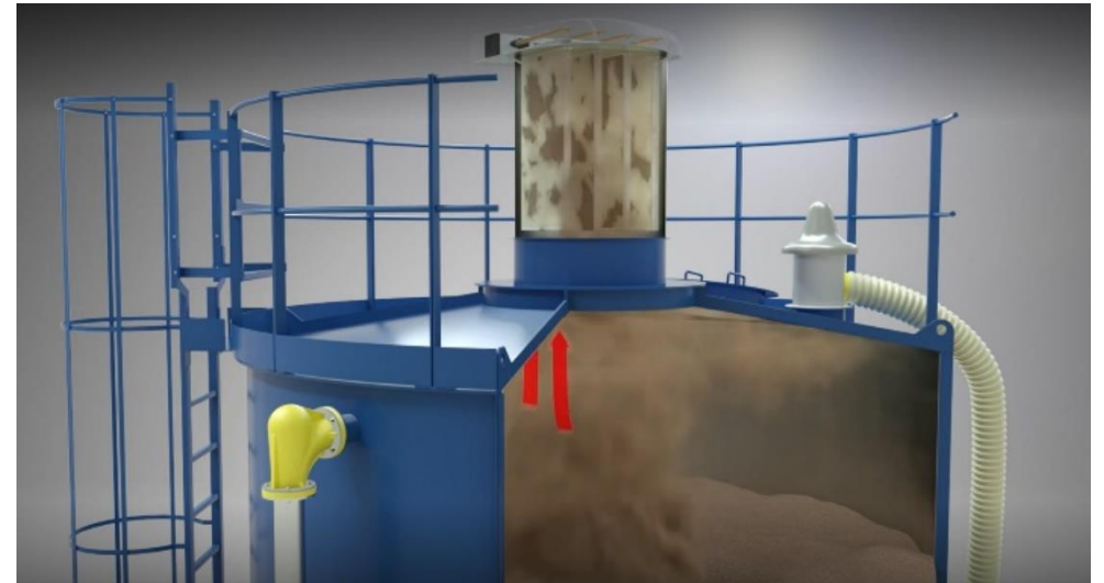
Video 8: Operation of silo venting filter including reverse-jet cleaning
