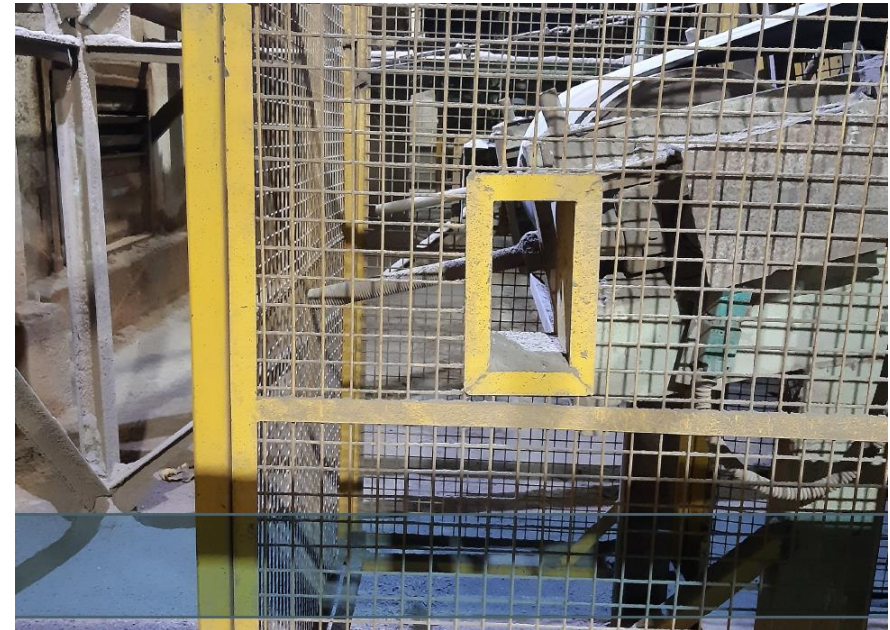
Picture 11: Examples of belt adjusters outside machine guard
