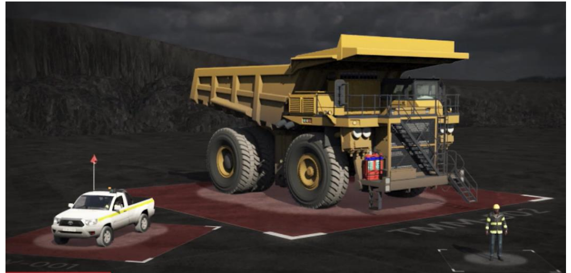
Video 21: Example of Collision Avoidance Technology – Mine Safe Pat System (PDG)
