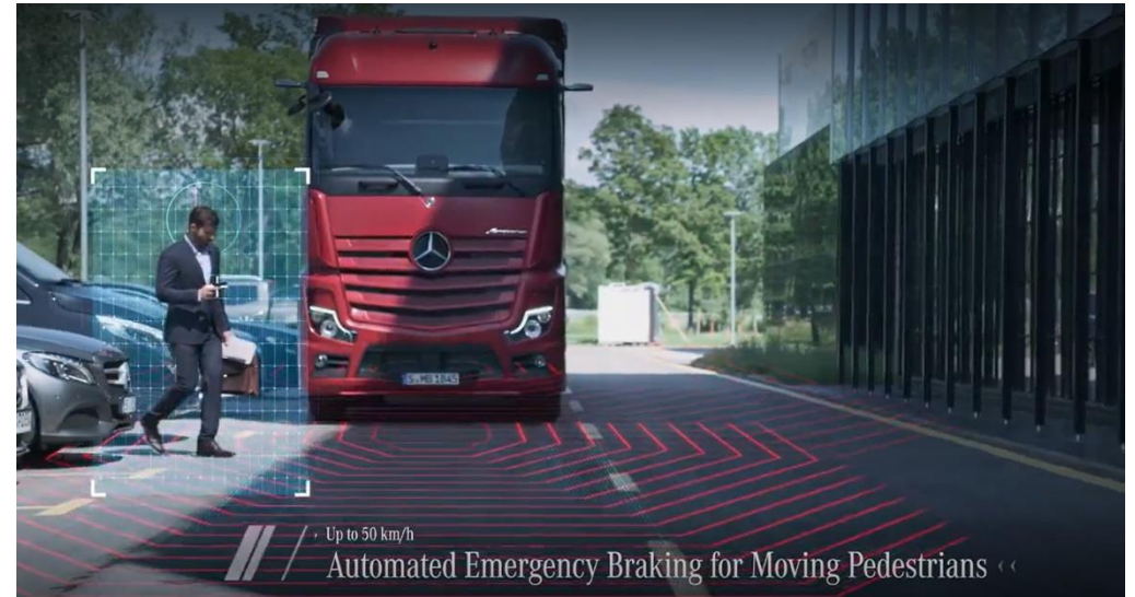
Video 43: Example of Advanced Emergency Braking System (Mercedes)
