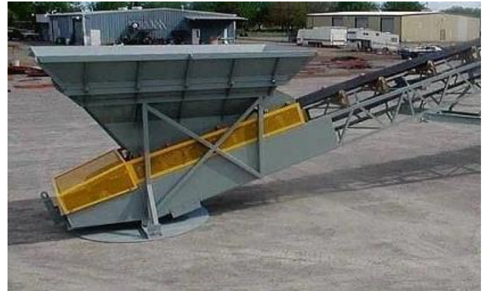
Picture 5: Example of Belt feeder guarding
