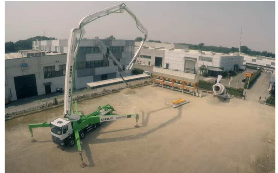
Video 71: Example of Pump Stability Control System – Smartronic (CIFA)
