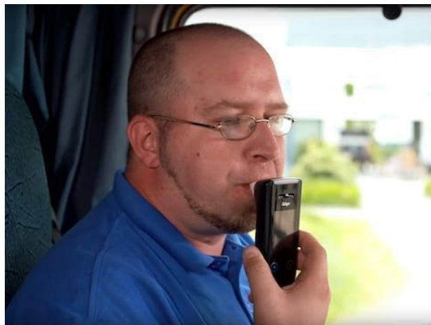
Video 74: Example of Alcohol ignition interlock (Dräger)
