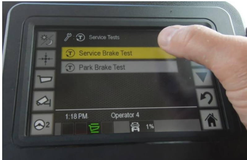
Picture 60: Example of Onboard Service Brake Test (Caterpillar)
