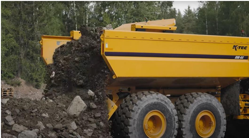
Video 24: Example of non-tipping dumper - Ejector Body (K-Tec)
