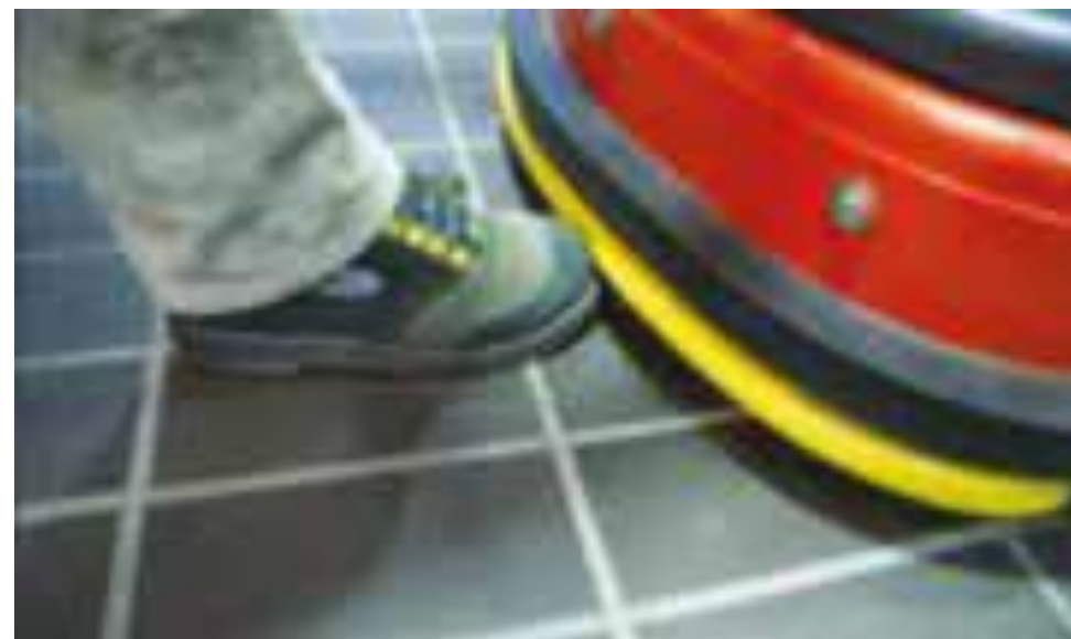
Picture 69: Example of active foot protection for electrical pallet truck
