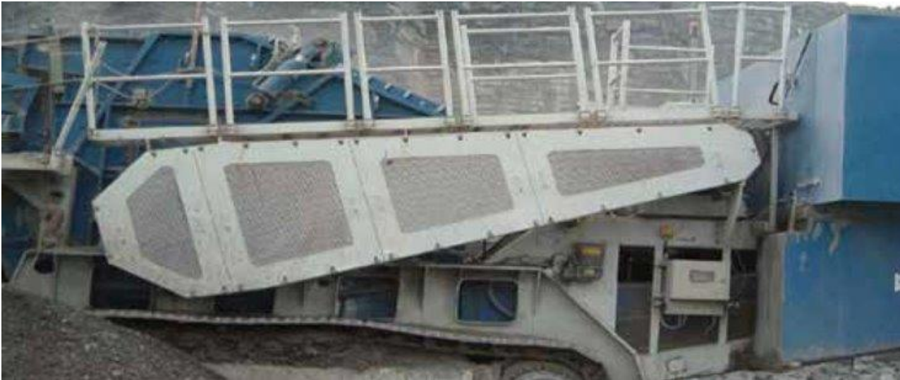
Picture 7: Examples of V belt guarding
