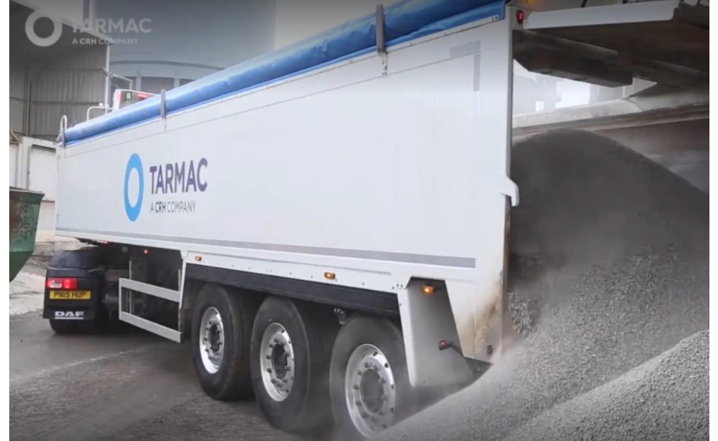
Video 54: Example of Non-tipping Trailer - Eliminating risk of vehicle overturn
