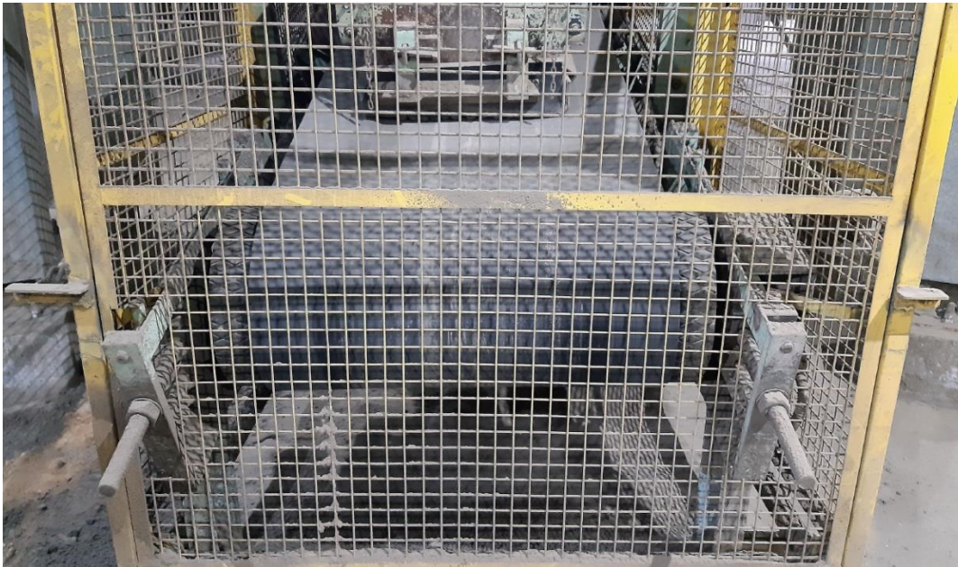
Picture 11: Examples of belt adjusters outside machine guard
