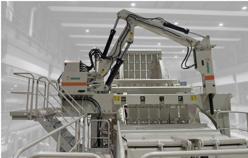
Video 6: Examples of remote-controlled rock breakers for fixed and mobile crushers
