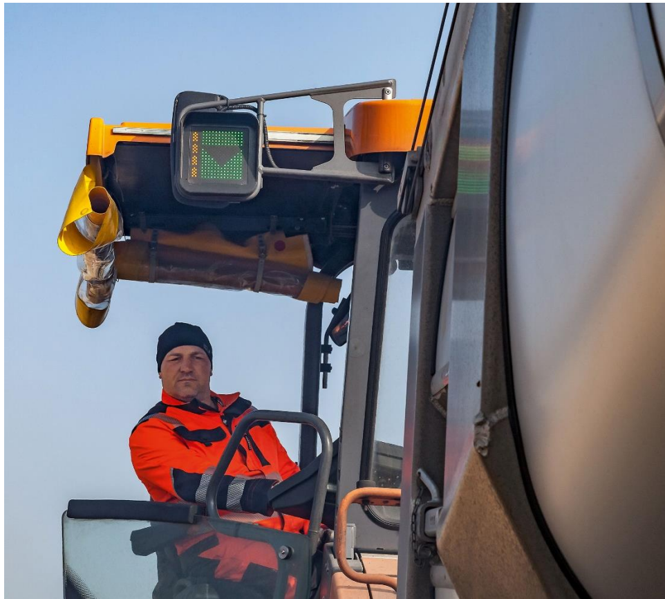
Video 38: Example of Traffic Light System - PaveDock Assistant (Wirtgen Group)
