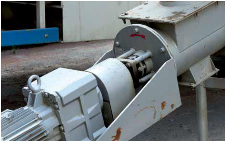
Picture 6: Example of skirting guard
