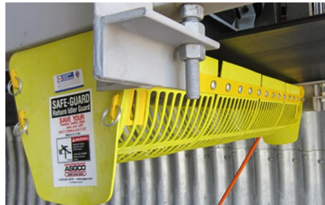
Picture 10: Examples of return roller guarding
