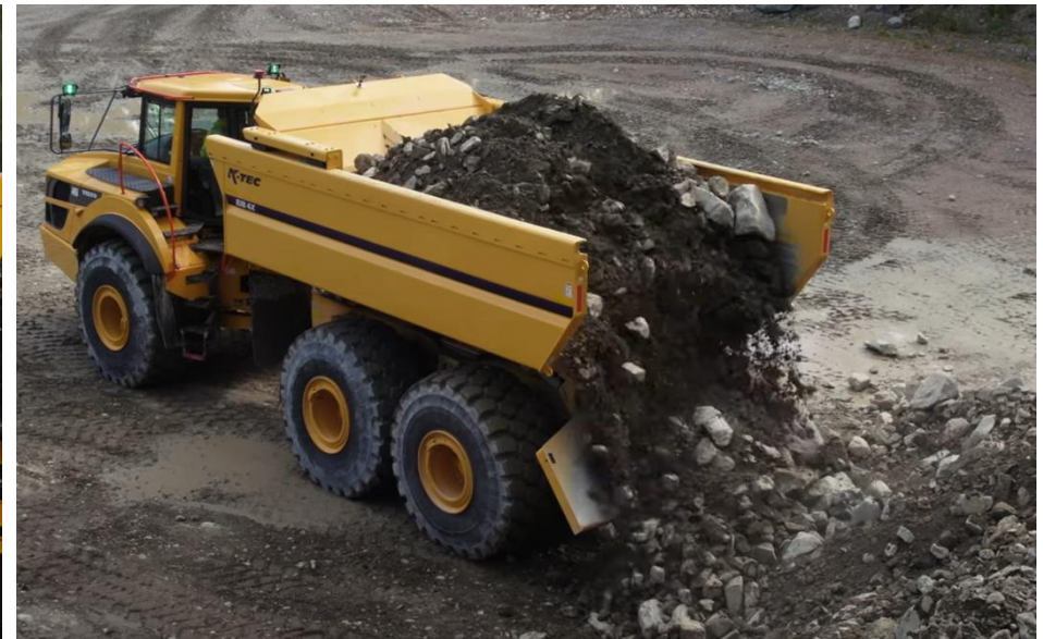
Video 24: Example of non-tipping dumper - Ejector Body (K-Tec)
