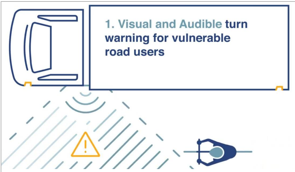
Video 48: Example of Side Audible Warning Alarm (Brigade)
