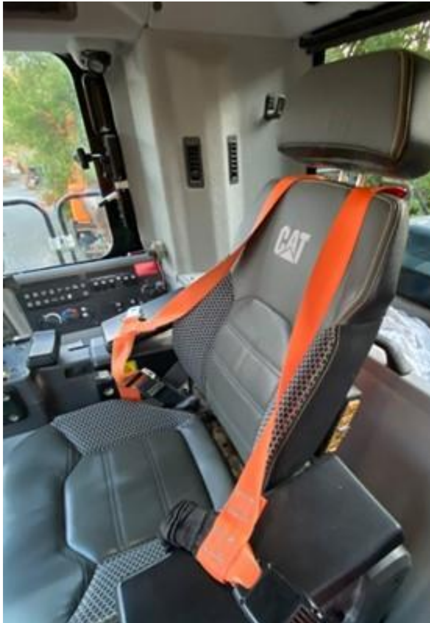
Picture 58: Example of high-visibility seat belt and seat belt use indicators – visual and audible dashboard alarm; a green light on the outside to indicate whether the safety belt is fastened
